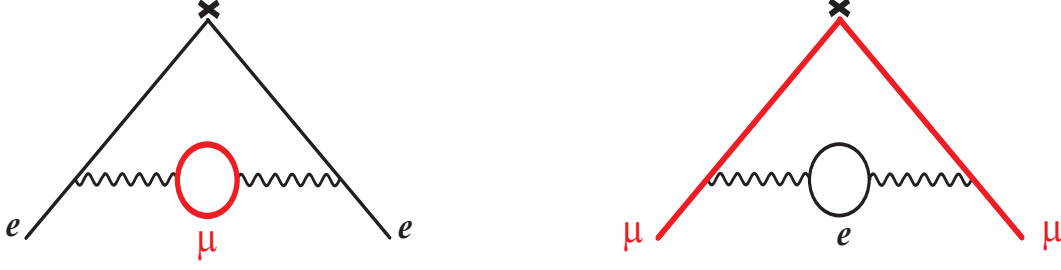
Figure 4: The insertion of a muon vacuum polarization loop into the electron vertex correction (left) or of an electron vacuum polarization loop into the muon vertex correction (right).
