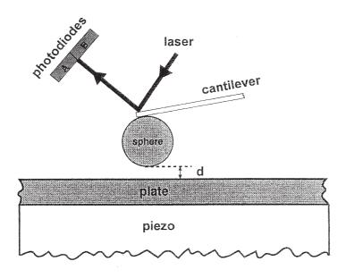
Figure 1: Experimental setup of the Casimir force measurement in [25, 26, 27]. The force is measured between the sphere and the plate with the distance of closest approach d (denoted L in the present report). The sphere is fixed on the cantilever of an AFM and its position measured by the deflection of a laser beam on the top of the cantilever. With kind courtesy of Umar Mohideen.
