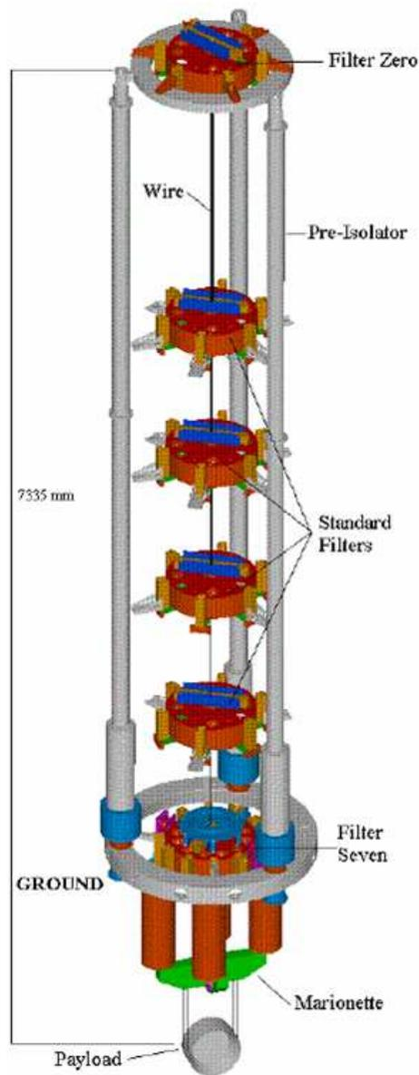
Figure 3: Superattenuator developed at Pisa
