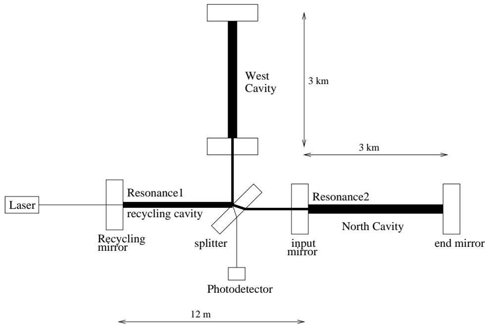
Figure 2: Sketch of a recycling Fabry-Perot interferometer
